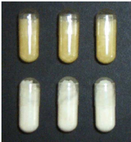
Fig. 7. Hard gelatine capsules directly filled with liquid hot PEG 1000 suspension (upper) and with granulated solidified PEG 1000 nanosuspension (lower) (with permission after [31]).
