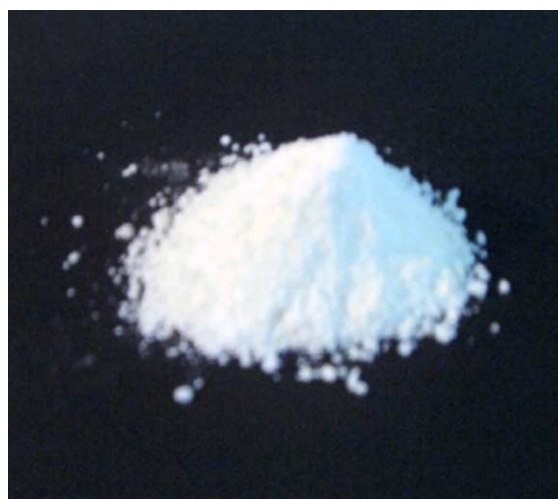
Fig. 6. Appearance of solid PEG nanocrystal dispersion after milling to a fine white powder (with permission after [31]).
